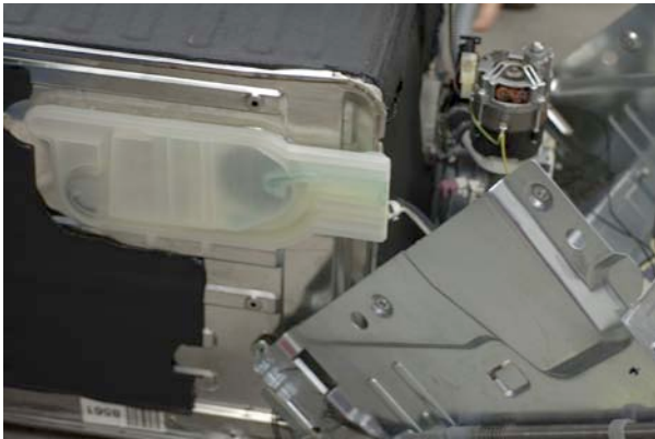
Airbreak softener mounted to tub
